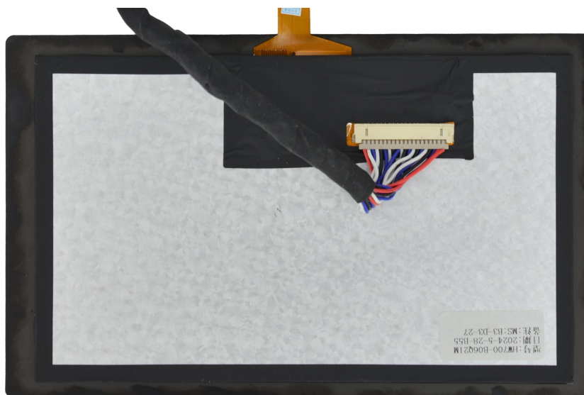
Figure 26 Connect LVDS screen cable to LVDS screen
